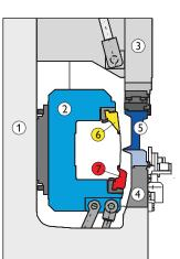
Two frames: the stationary main frame (1) of the machine and a C-frame (2) with hydraulically actuated swinging movement up-wards or downwards.
